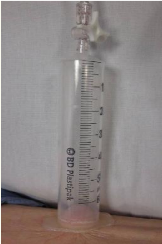
Fig. 1. Syringe connected to wall suction at -200 mmHg.
