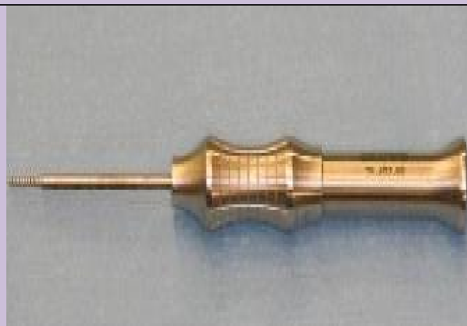
Fig. 1. Repositioning pin placed in the handle of a miniscrewdriver.
