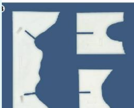
Surgical template consisting of 3 parts constructed with Catia. Horizontal templates can be plugged into the vertical template. Small flanges prevent unintentional mobility. Note, L imprinted on left side as a help for correct assembly.
